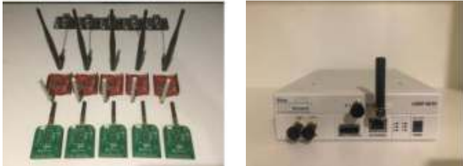
Figure 9: LoRa transceivers and USRP SDR
