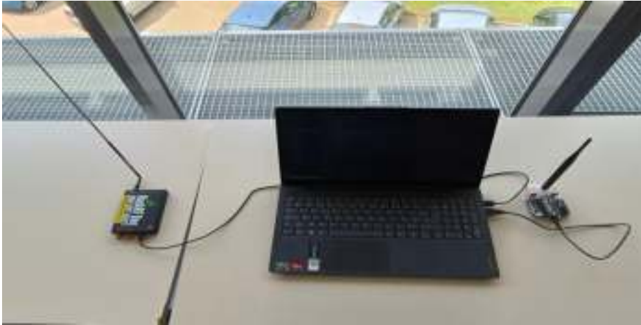
Figure 6: LoRa transceivers and HACKRF SDR
